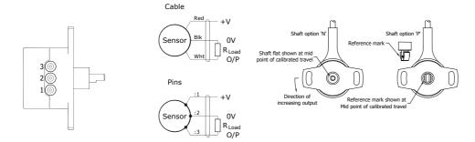
**Mechanical Mounting:** Flange mounted. The flange slots are 4.5mm by 20 degrees wide, 48mm pitch. The sensor should be mounted with minimal axial and radial loading on the shaft for optimum life. It is recommended that the shaft is coupled to the drive using a flexible coupling. Option 'N' shaft: Ø 4 mm x 8 mm long, flat 3 mm A/F x 4 mm. Option 'P' shaft: fits 6 x 3 mm slot.
